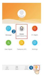
2. Connect to the inverter WiFi. Log in as **installer**, and perform **Quick settings**.
