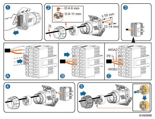
**Step 2** Connect the signal cable to the COM port.
