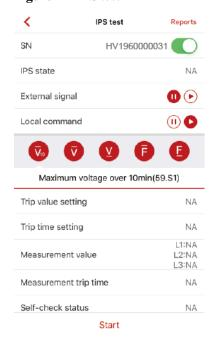
**Step 2** Choose to start the S1 or S2 check as required. The default check type is S2. To start the S2 check, you need to set **External Signal** or **Local Command**.
