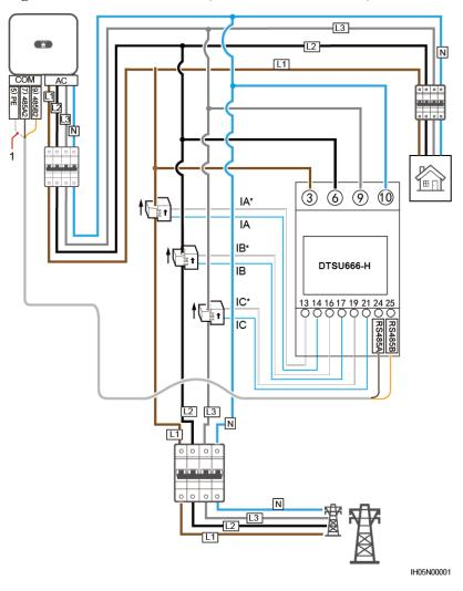
Figure 5-23 Cable connection (Three Phase Four Wire)
