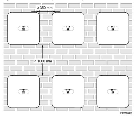
Figure 4-5 Stacked installation (not recommended)
