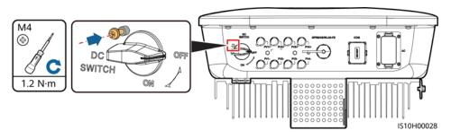
Step 5 Turn off the DC switch between the SUN2000 and PV strings.
