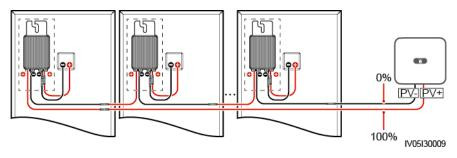
Figure F-2 Definition of the percentage of the short-circuit position
