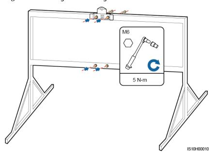
Step 4 Install the SUN2000 onto the mounting bracket.
